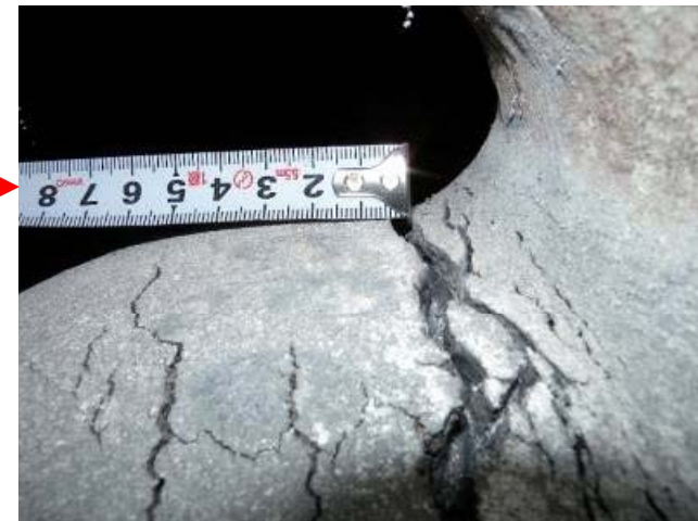
Lead damper and crack on the surface
